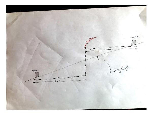
The top part to the right of the red partition would be plan A (910x500) if we do not have enough money to build the entire structure at once. It would have a concrete tiled floor and bamboo structure and would include the kitchen, bathroom, storage room and our bedroom. The bedroom would be separated from the adjoining kitchen by a bar counter, with an optional moveable partition if we wanted privacy.
