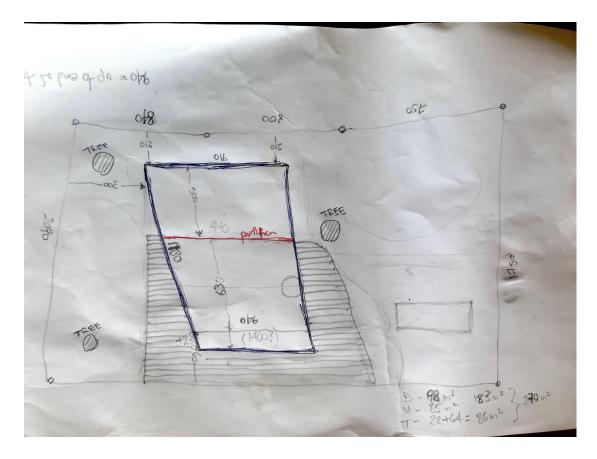
The red partition is in case we cannot borrow enough money to build the entire structure at once, so we could start with an area of about 910x500 (top half).
